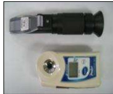
Refractometer, analog (top) and digital (bottom)
