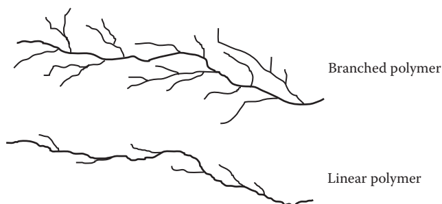
FIGURE 2.5 Schematic representation of branched and linear polymers showing the larger volume swept out by the branched structure, resulting in its lower density. Branches of the main backbone are indicated by narrower lines; they have no direct proportional relationship to cross-sectional dimensions. (From Brown, W.E., Plastics in Food Packaging: Properties, Design and Fabrication , Marcel Dekker, New York, p. 106, 1992.)
